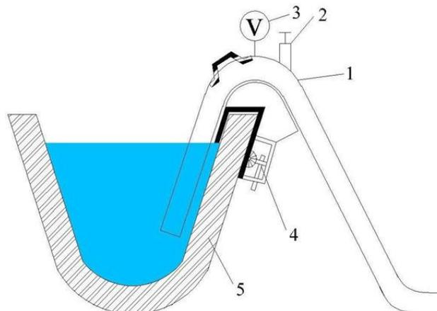
**Figure 2.** Scheme of the siphon pipe: 1-siphon pipe; 2-air release pouch; 3-vacuum meter; 4-tray; 5-screw
