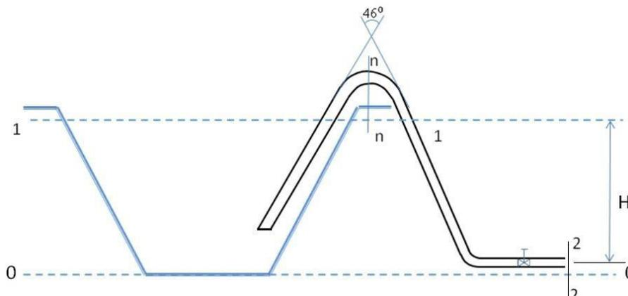
**Figure 1.** Calculation scheme of siphon device
