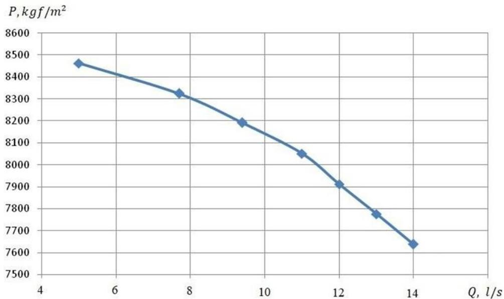
**Figure 3.** Graph of  $Q=f(P)$  to determine water discharge
