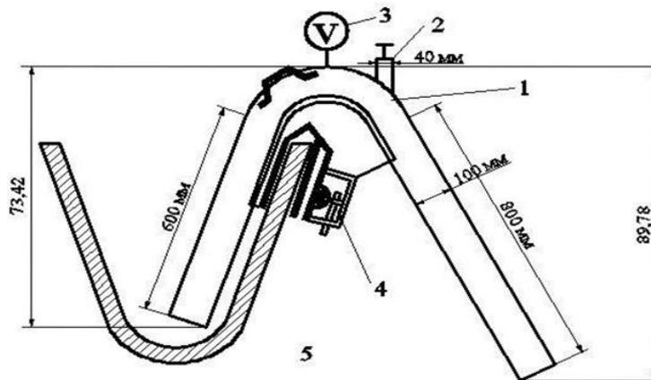
**Figure 4.** Portable siphon water meter
