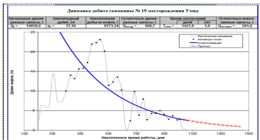
Figure 2. Dynamics of flow rate of well No. 19 of the Umid field (graph built in MS Excel)
