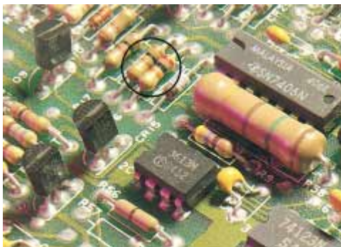
Figure 27.6 The colored bands on a resistor represent a code for determining resistance. The first two colors give the first two digits in the resistance value. The third color represents the power of ten for the multiplier of the resistance value. The last color is the tolerance of the resistance value. As an example, the four colors on the circled resistors are red (= 2), black (= 0), orange (= 10^3 ), and gold (= 5%), and so the resistance value is 20 \times 10^3 \Omega = 20 \text{ k}\Omega with a tolerance value of 5% = 1 k \Omega . (The values for the colors are from Table 27.2.)
