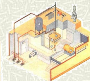
Above: India's sludge irradiation research facility in Baroda. As shown in the schematic, the facility includes the irradiation cell (1); storage silo (2); irradiation vessel (3); source assembly (4); pump house (5); recirculation lines (6); obnoxious gas exhaust (7); transport container (8); control console (9); and source coolant system (10).
