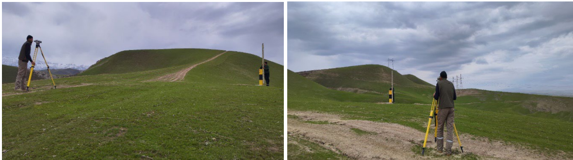
Figure 3. Installation of new geodetic stations during network densification activities in the Fergana Valley.
