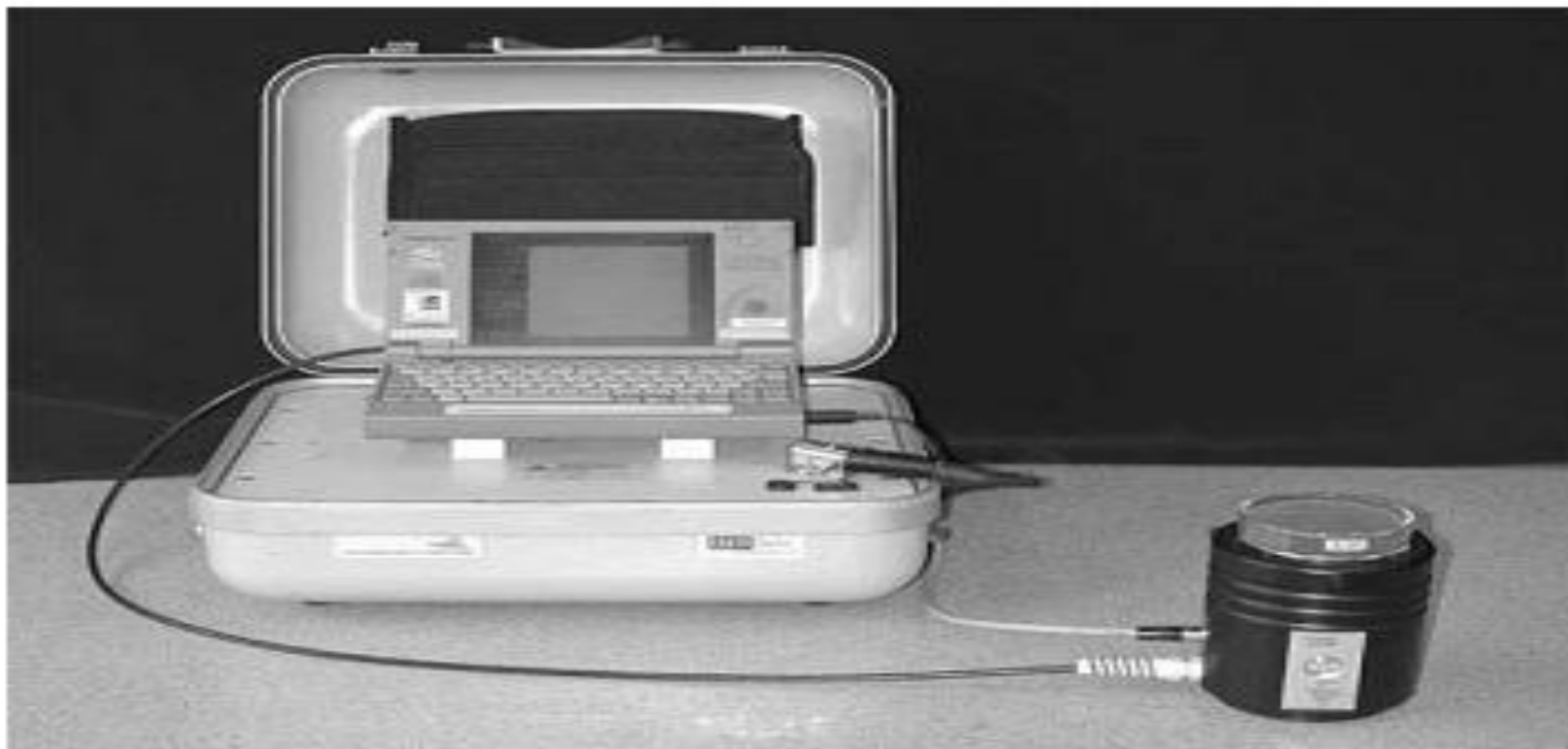
Fig. 1 Portable visible–near-infrared spectrometer being used to scan a soil sample contained in a petridish. With this setup 500 samples per day can be routinely scanned. ( View this art in color at www.dekker.com . )
