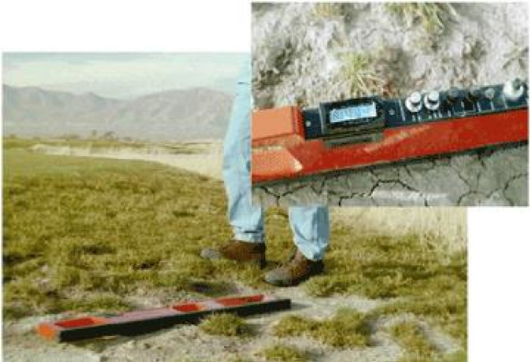
A portable electromagnetic (EM) soil conductivity sensor used to estimate the electrical conductivity in the soil profile
