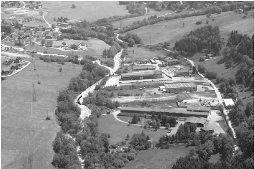
Fig. 6 Industrial and commercial settlements of an Alpine valley in the Central Alps. The buildings through the alluvial riverbed and obstruct the discharge of the almost ten-yearly floods. Arrows indicate the direction of the river flow (Photo by courtesy of IRPI-CNR)
