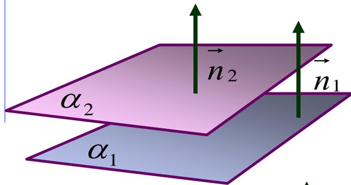
$$\vec{n}_1 \parallel \vec{n}_2 \Rightarrow \frac{a_1}{a_2} = \frac{b_1}{b_2} = \frac{c_1}{c_2}$$
