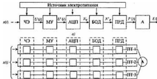
Picture 1. Functional diagram of a mobile device for collecting data from an environmental monitoring system
