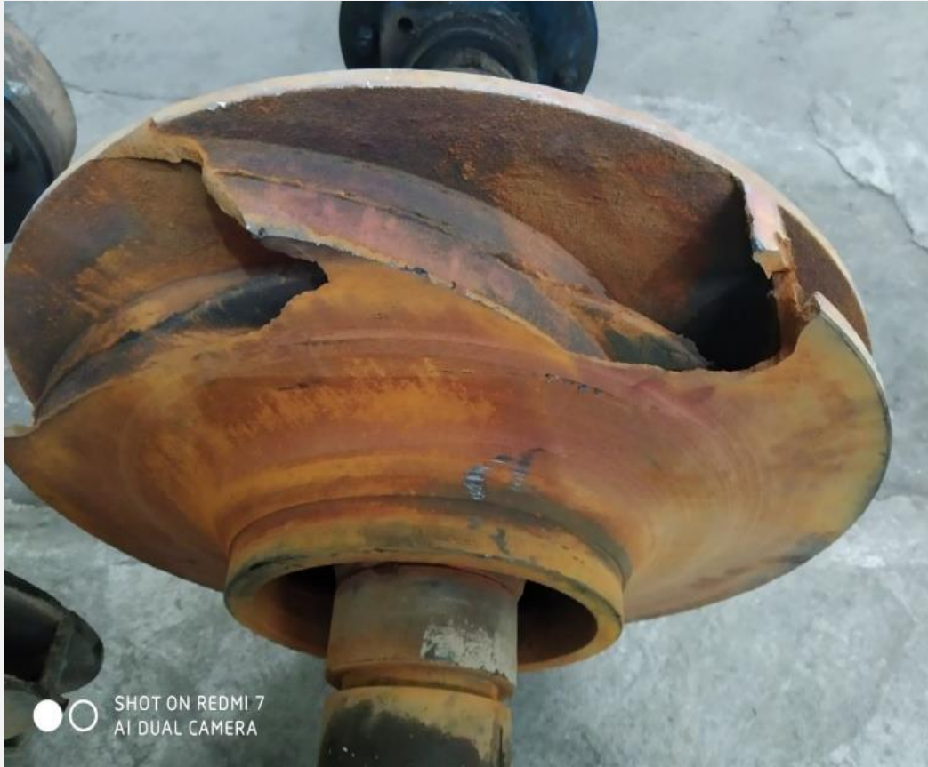
Figure 1. "D" type pump impeller collapse occurred as a result of cavitation and disruption of water flow dynamics
