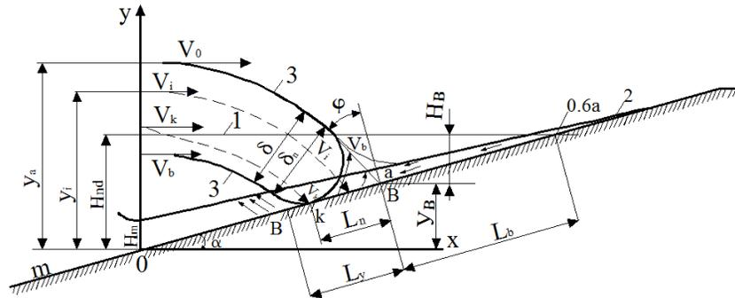
**FIGURE 2.** Kinematic scheme of the impact generated by the reference barrier:
