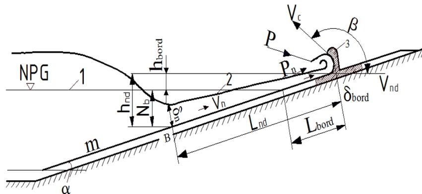
**FIGURE 4.** Diagram of the dynamic forces of water flow to the wall
