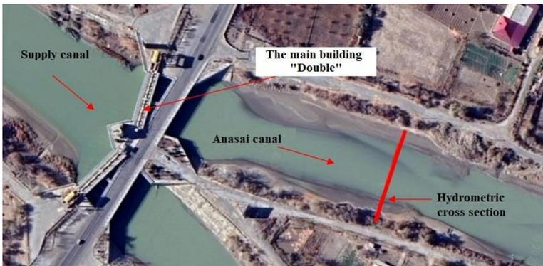
**Fig. 2.** Plan of the head structure of the Anasai canal and the location of the site for the hydrometric measure
