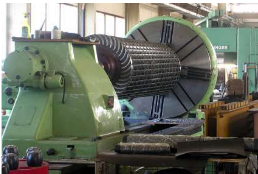
8.54-rasm. Ikki karra harakatlanadigan turbinaning rotori
