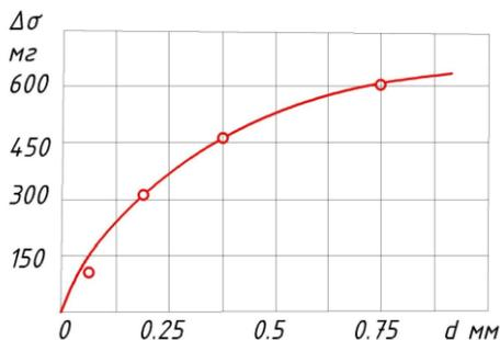
**Fig. 1.** Influence of fineness of deposits on the value of hydroabrasive wear of the blades of the impeller of a centrifugal pump.
