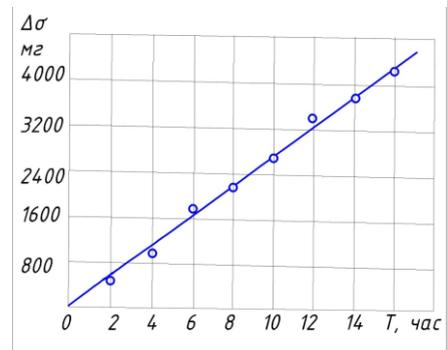
**Fig. 2.** The dependence of the intensity of wear of the impeller blades on the duration of the centrifugal pump
