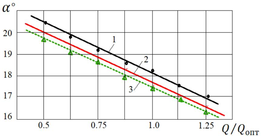
**Fig. 5.** Influence of the operating mode of a centrifugal pump on the interaction  $\alpha$  of a solid particle with the surface of the blade: 1-3, respectively, for the middle and end parts of the blade, 2, for the radius  $R = 0.75 \cdot R_2$
