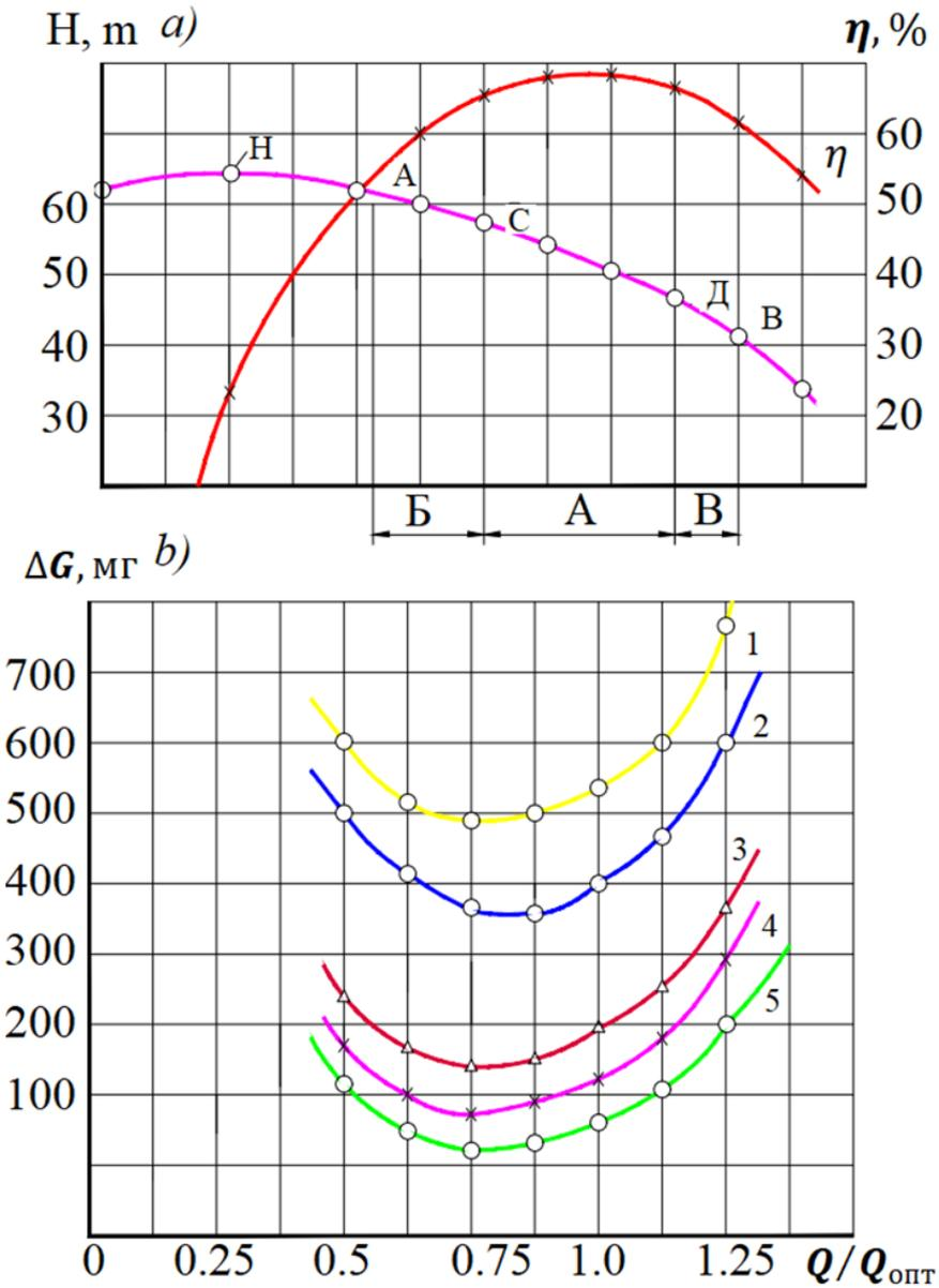
**Fig. 3.** The intensity of wear of the impeller blades from the operating mode of the centrifugal pump 3K-6 ( $n_0 = 2900$  rpm): *a* is pump characteristic, *b* is wear of blades made of various materials; 1 is silumin, 2 is ferromanganese with epoxy resin, 3 is steel (St. No. 3) 4 is monocorundum with epoxy resin, 5 is silicon carbide with epoxy resin.
