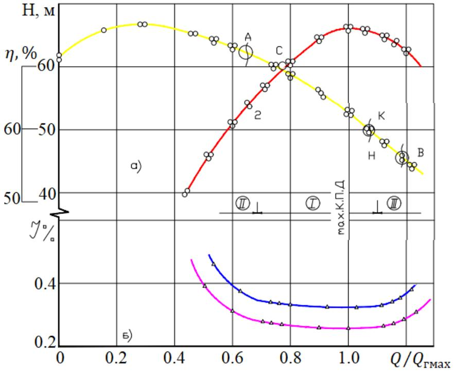
**Fig. 4.** Influence of the operating mode on the intensity of hydroabrasive wear of the impeller of a centrifugal pump 4K-8 ( $n_0=2900$  rpm): *a* is pump characteristic, *b* is wear of the blades.
