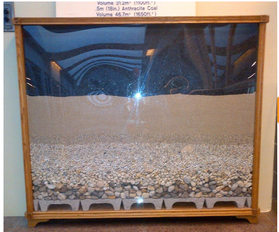
This is a diagram cross-section of the filters present at Elgin and Huron treatment plants.
