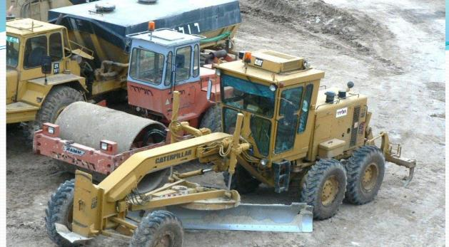
• Graders are commonly used in the construction and maintenance of dirt roads and gravel roads. In the construction of paved roads they are used to prepare the base course to create a wide flat surface upon which to place the asphalt. Graders are also used to set native soil foundation pads to finish grade prior to the construction of large buildings.
