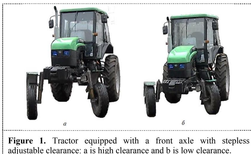
**Figure 1.** Tractor equipped with a front axle with stepless adjustable clearance: a is high clearance and b is low clearance.
