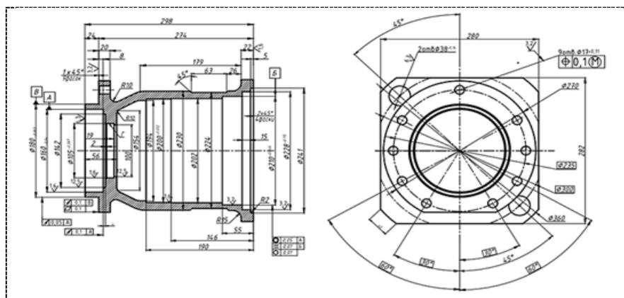
**Figure 4.** The holder of the mechanism for changing the clearance of the rear axle.
