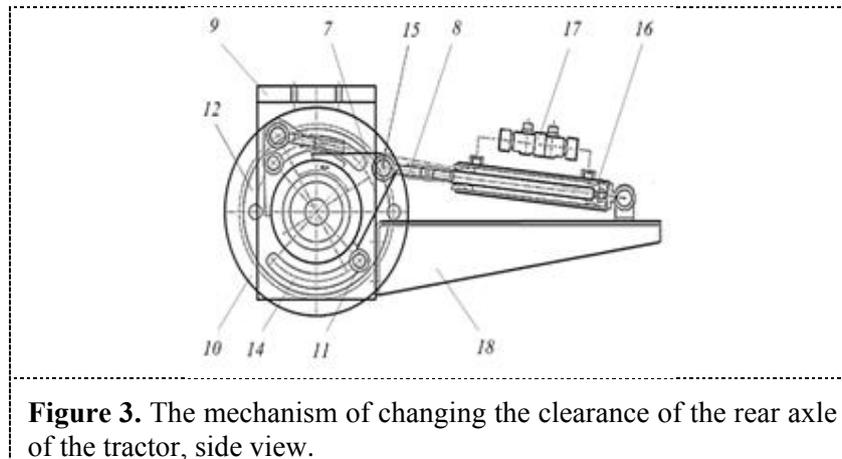
**Figure 3.** The mechanism of changing the clearance of the rear axle of the tractor, side view.
