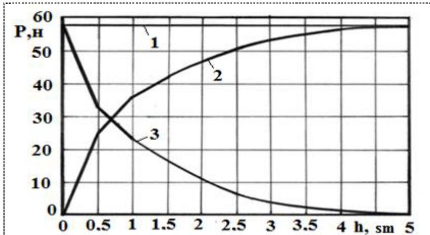
Figure 3. The force on the blade of the knife with various values of preliminary bends lower than the limiting  $f_{max} = 5.85 \text{ sm}$
