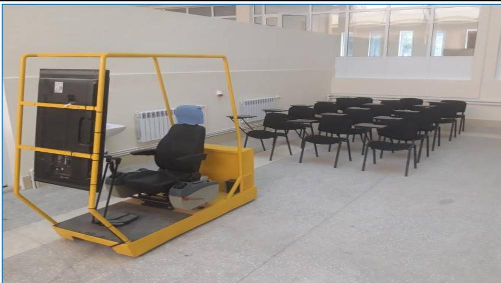
Figure 2. "Excavator simulator" based on a bucket excavator.
