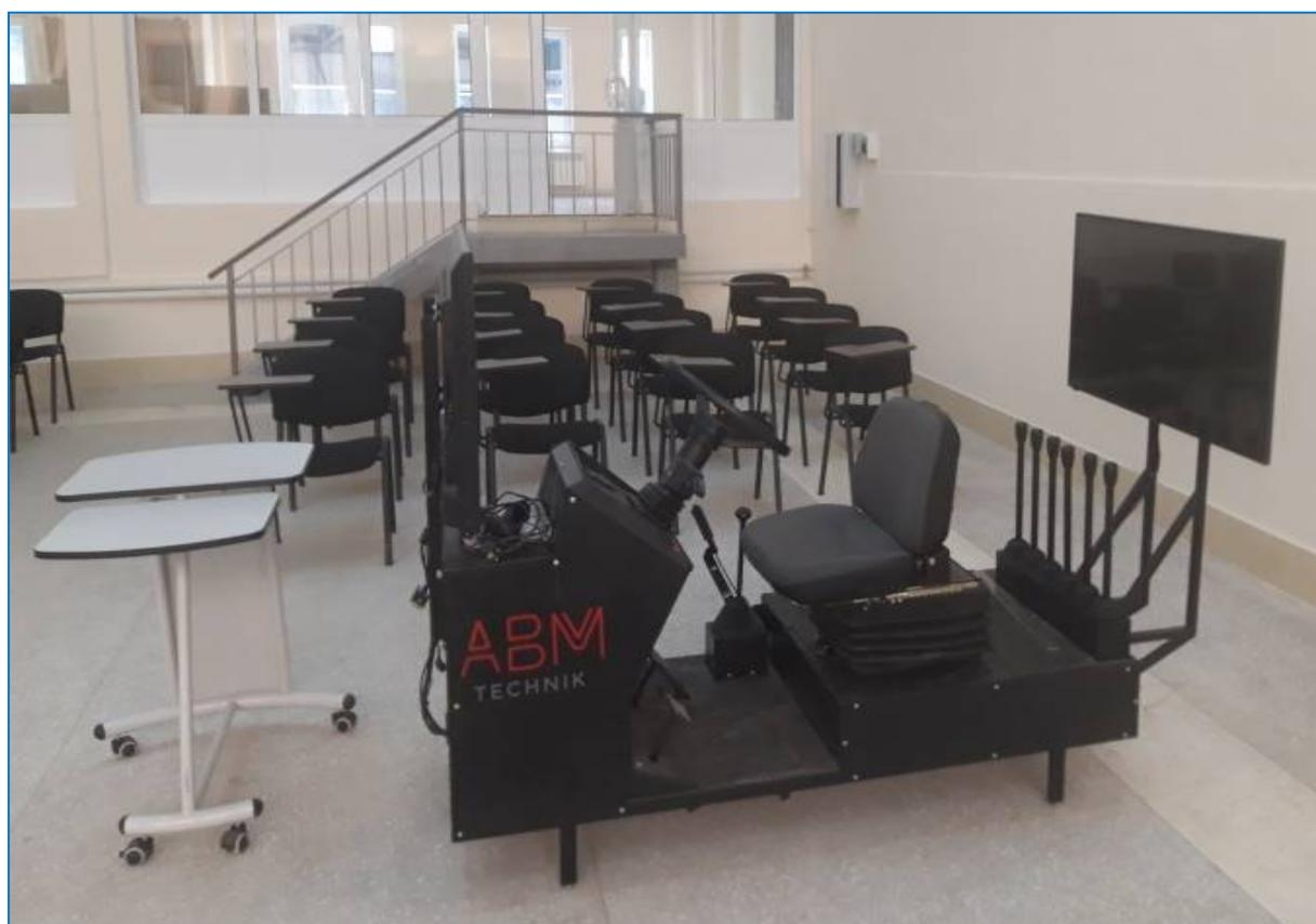
**Figure 1. "Universal tractor simulator" based on MTZ tractor.**
