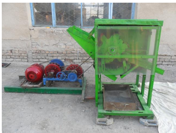
Figure 1. A device for laboratory to observe the peeling process of the corn-cob
