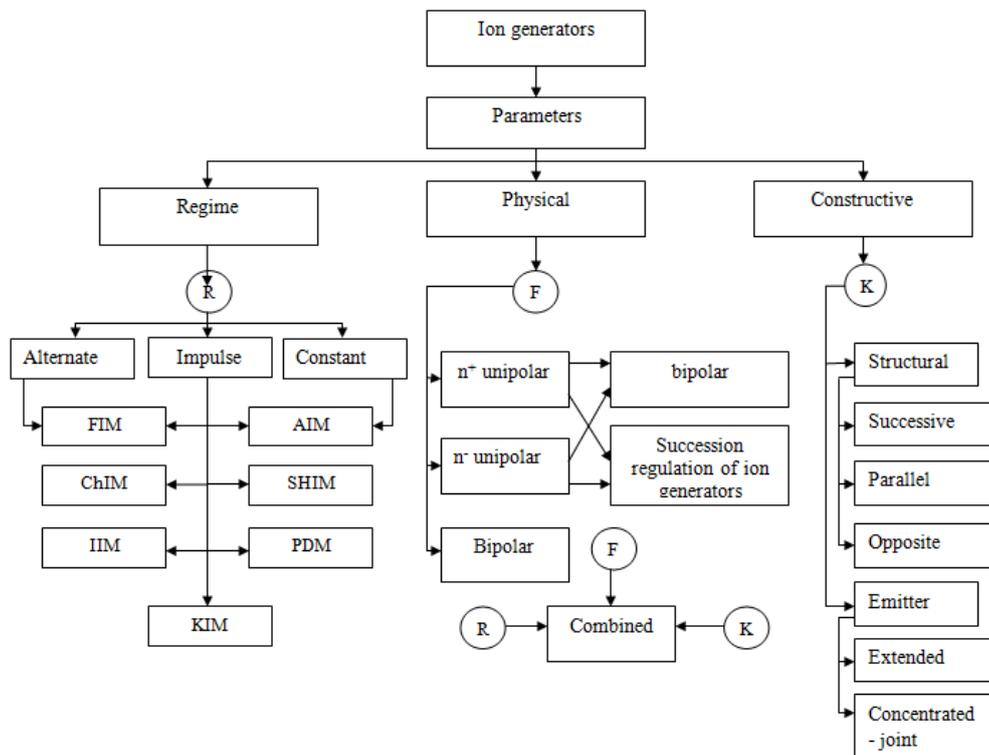
**Figure 1.** Classification of corona discharge ion generators
