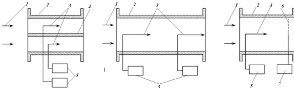
**Figure 2.** Block diagrams of corona ionizers switching: a) parallel; b) successive; c) opposite 1 - air flow; 2 - air duct element; 3 - corona electrodes; 4 - baffle wall; 5 - high voltage sources; 6 - control grid, ring or filter; 7 - control electrode power supply
