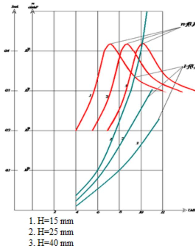
**Figure 3.** Volt-ampere and volt-ion characteristics of the ion generator at various distances of the discharge gap
