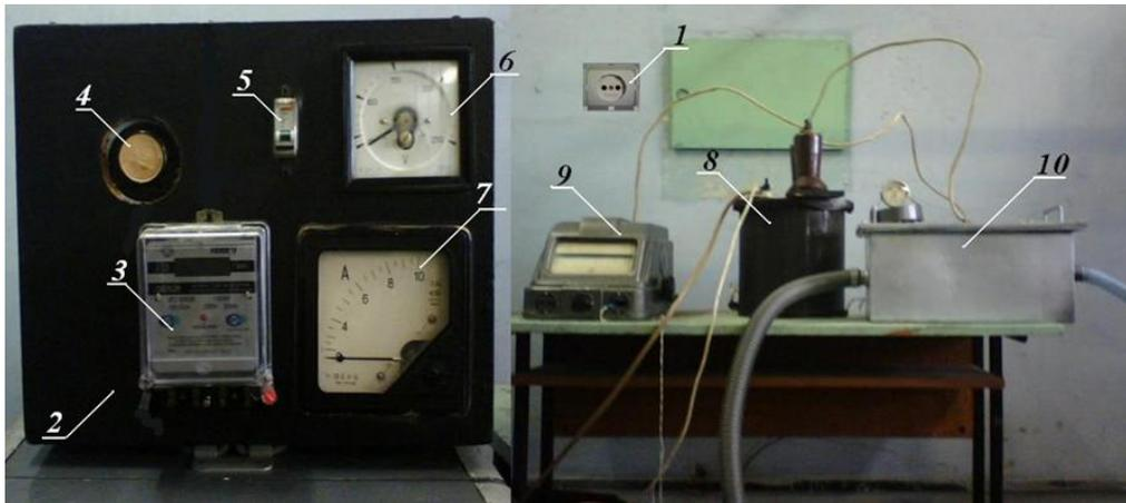
**Figure 1.** 1 – 220 V power supply; 2 – control unit; 3 – one-phase electricity meter; 4 – autotransformer; 5 – automatic switch; 6 – 230 V voltmeter; 7 – 1 A ammeter; 8 – 10 kV transformer (NOM 10); 9 – 10 kV kilovolt-meter; 10 – ozone generator
