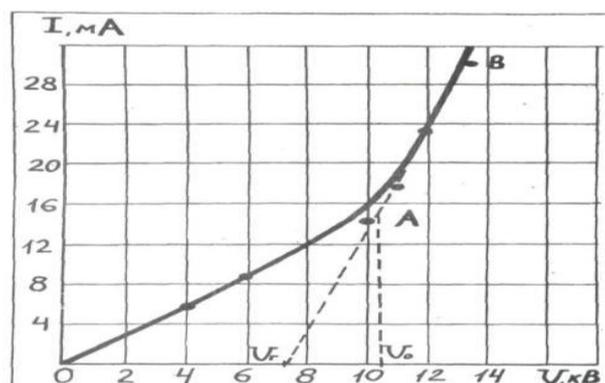
**Figure 2.** Volt-ampere characteristic of ozone generator
