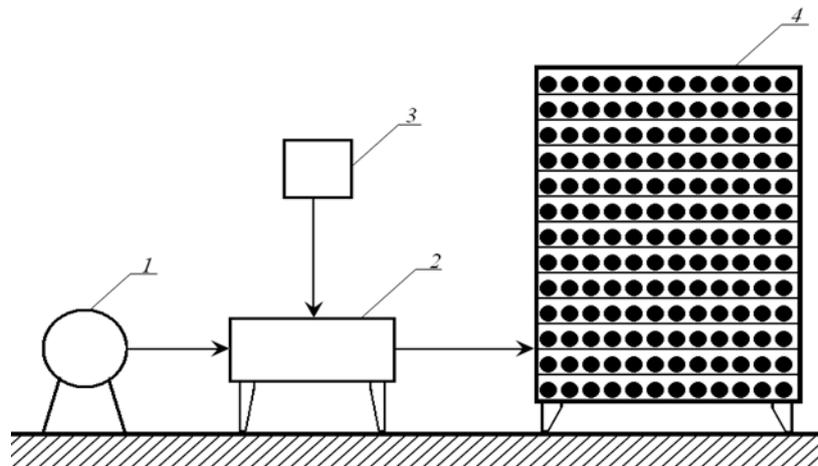
**Figure 4.** Supplied ozone-air mixture from the generator to the storage: 1 – compressor, 2 – ozone generator, 3 – power supply, 4 – treatment chamber
