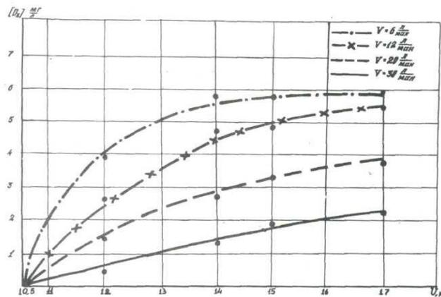
**Figure 3.** Dependence of the ozone volume on the applied voltage and air flow
