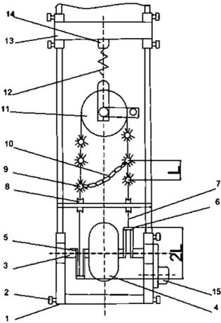
**Fig. 1.** Device for cleaning gutters (top view): 1-mounting frame; 2-clamp; 3-shaft; 4-water wheel; 5-eccentric; 6-portable wallpaper; 7-thin wire; 8-blocks; 9-softeners; 10-wheel; 11-drum; 12-spring; 13-frame; 14-mobile pin; 15-mechanical drive.
