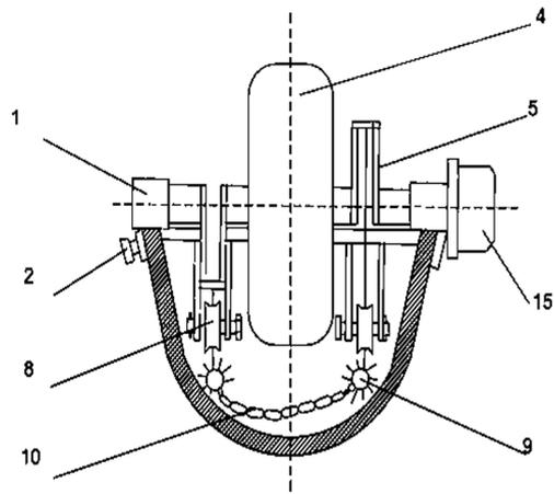
**Fig. 2.** Device for cleaning gutters (side view): 1-mounting frame; 2-clamp; 4-water wheel; 5-eccentric; 8-blocks; 9-softeners; 10-chain; 15-mechanical drive.
