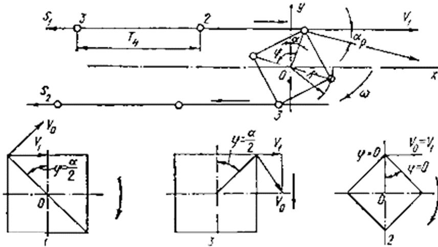
**Fig. 3.** Scheme of the chain movement along the star.
