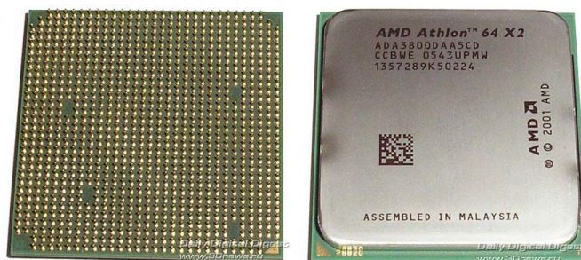
5.7-rasm. Socket M2 uchun AMD protsessori
