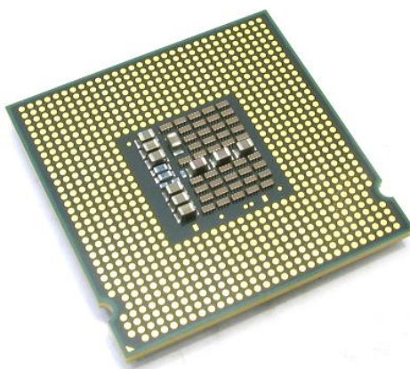
5.6-rasm. Socket LGA775 uchun Intel protsessori
