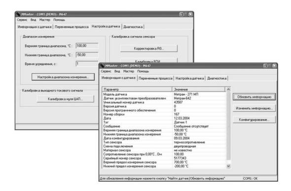
The program is designed for configuration and setup of Metran-270MP Smart Temperature Transmitter (further transmitter) complete with the normalizing converter.
