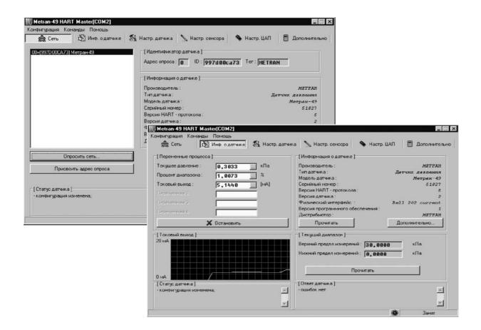
H-Master Software is designed for setting Metran-100, 3051S/T, 3051S Smart Pressure Transmitters, Metran-280, 248 Smart Temperature Transmitters, Metran-300PR Flowmeters and other HART devices. The program has user-friendly interface.
