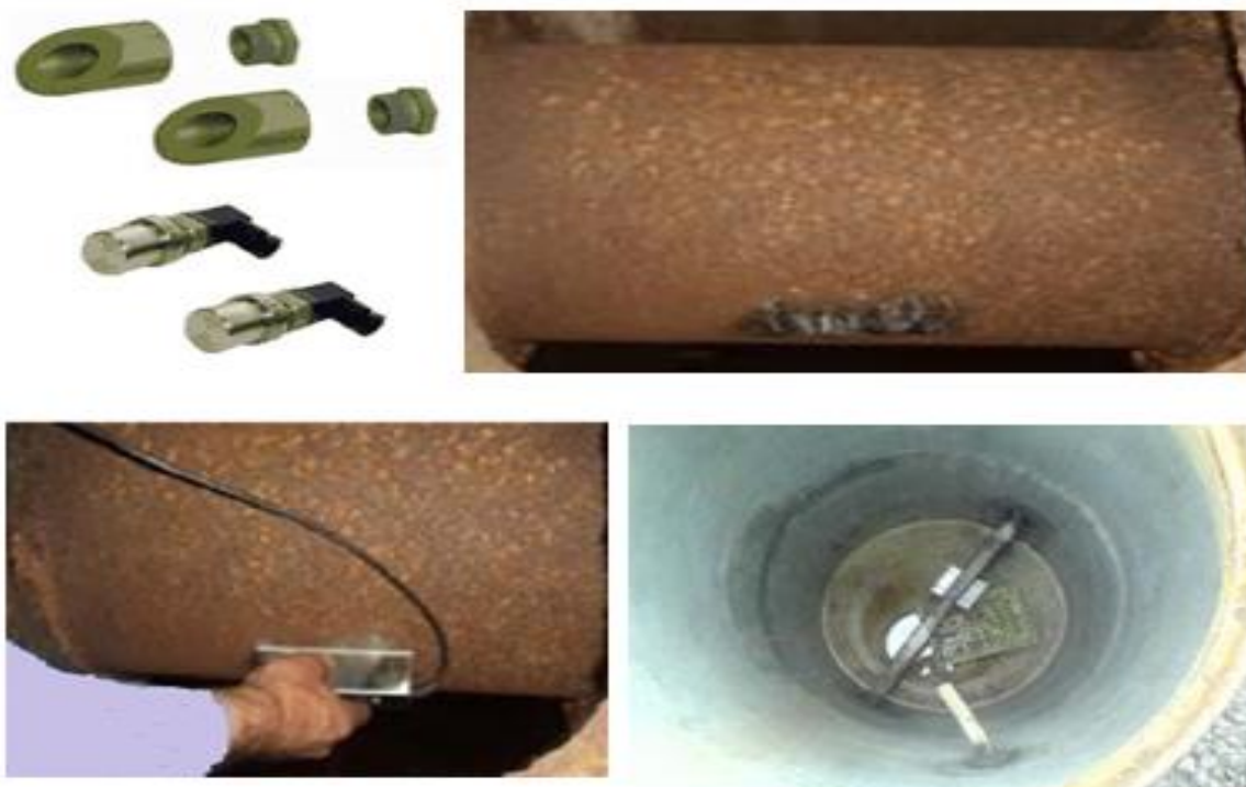
11.4-rasm. Datchikni quvurga o`rnatish
