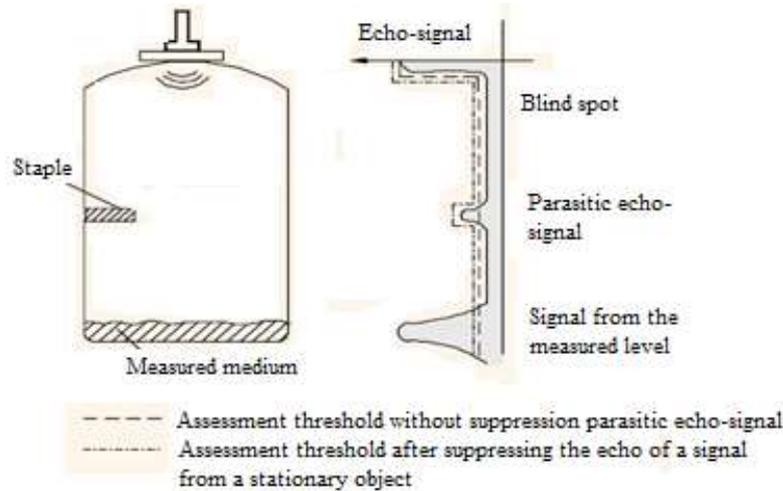
Fig. 3. Suppression of an echo - signal from a stationary object in the tank.
