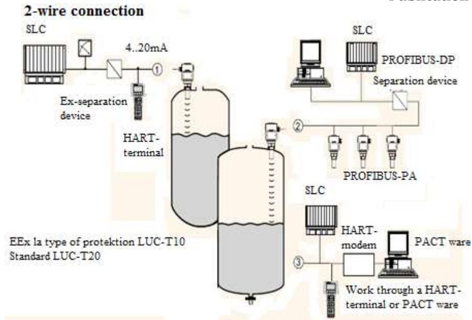
Fig. 4. Installation and connection methods for ultrasonic sensors of the LUC-T series.
