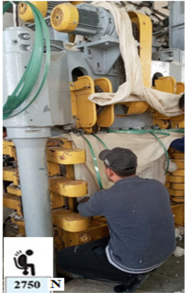
3-rasm. O'tirib ishlashda gavda holatiga tushadigan kuch.
