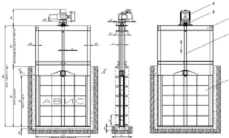
**Figure 1.** Structural diagrams of the gear and linear electric drive of a flat gate: 1 - watergate; 2 – gate rod; 3 - frame; 4 - inductor of a linear cylindrical induction motor; 5 - fixing mechanism.
