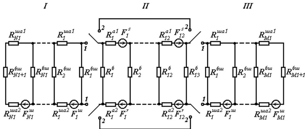
**Figure 3.** The equivalent circuit of the magnetic circuit of the machine: induction converter with an open magnetic circuit - closed contacts 1; (I, III) - shunt zones, II - inductor core zone; Inductive converter with a closed magnetic circuit - closed contacts 2.
