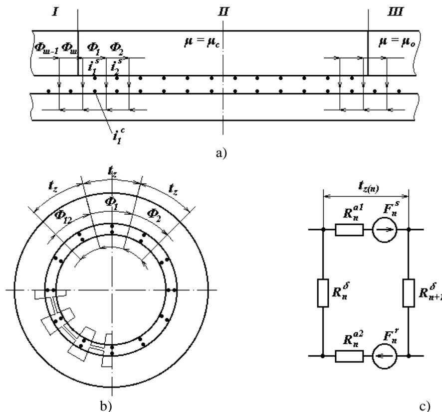
**Figure 2.** The design model of the magnetic circuit: a - the magnetic circuit is open, (I, III) - shunt zones, II - the core zone of the inductor; b - the magnetic circuit is closed; c is the equivalent circuit of the  $n$ th section.
