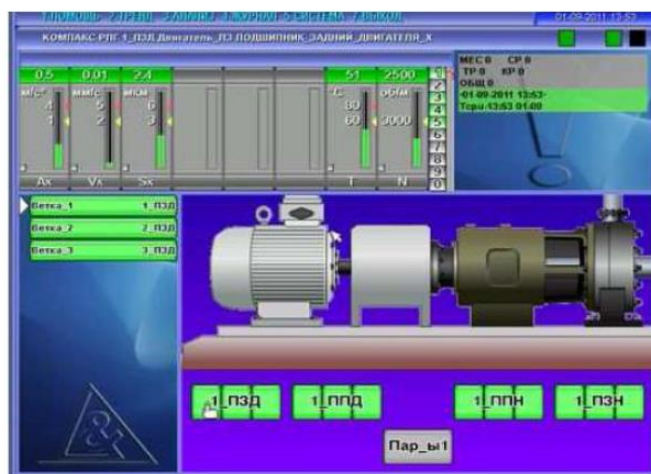
1 pic. Screen of the diagnostic station in the "MONITOR" mode
