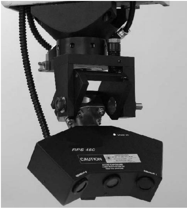
Figure 1 A laser scanner may be attached to a mechanical actuator to increase its work volume. (Photograph courtesy of Laser Design Inc., Minneapolis, MN.)
