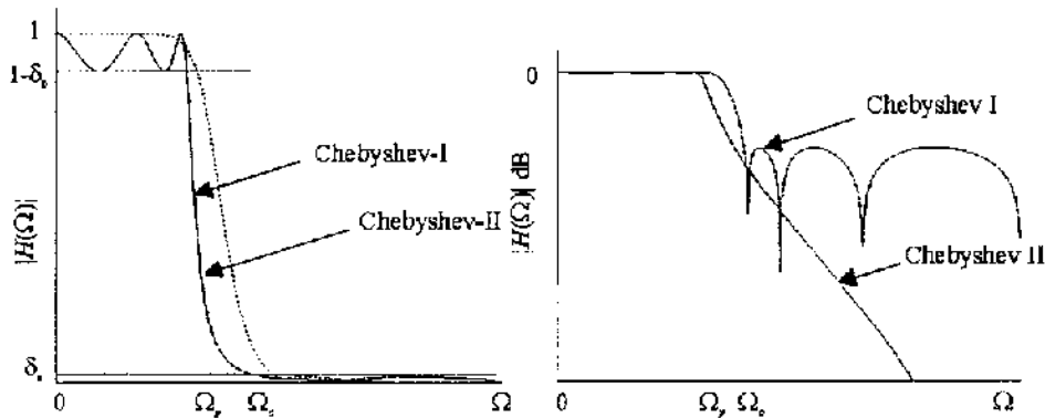
Figure 10 Typically Chebyshev-I and -II lowpass filter magnitude frequency response (linear on the left, logarithmic on the right).
