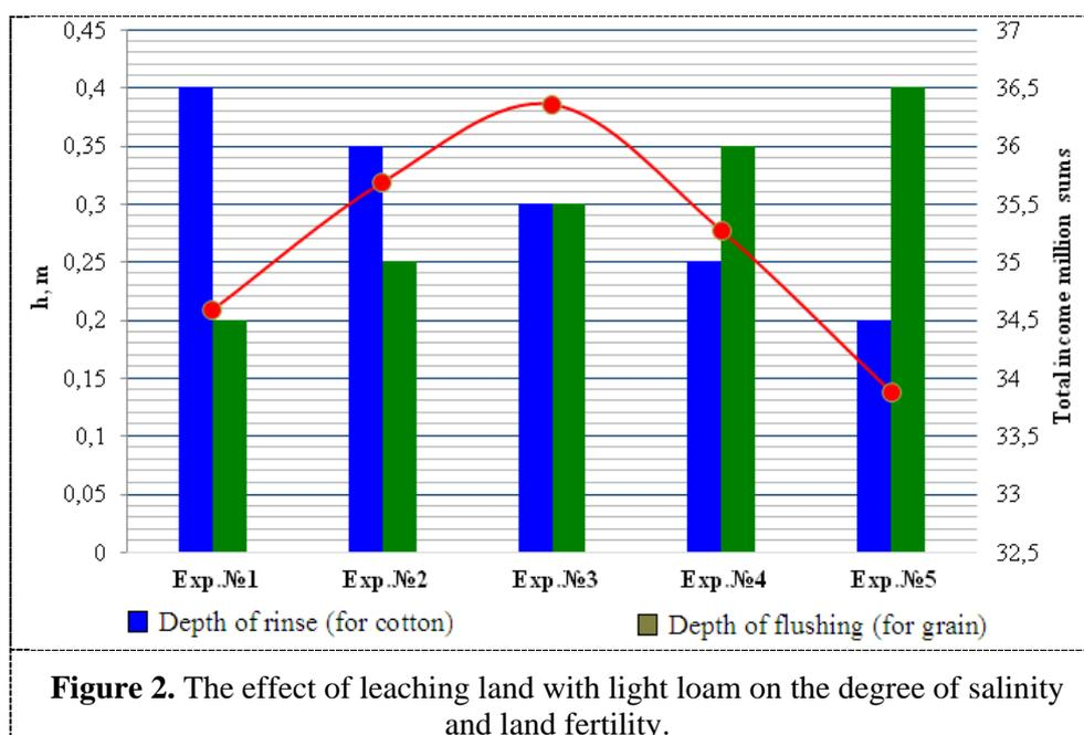
It can be seen from figure 2 that if the leaching norm is used taking into account the plant species, i.e. for the sowing of cotton, the flow of water is 4000 m<sup>3</sup>/ha and for corn 2000 m<sup>3</sup>/ha, in this case, the yield of crops is not high. But, if you do not change the water consumption for land leaching in these areas, i.e. for the field with cotton planting to use 3000 m<sup>3</sup>/ha and for corn 3000 m<sup>3</sup>/ha, the relatively average crop yields increase.
