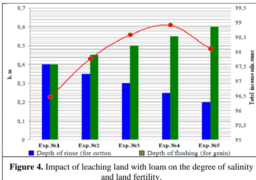
It can be seen from Fig. 4 that if the leaching norm is used taking into account the plant species, i.e. For the sowing of cotton, the flow of water is 4000 m<sup>3</sup>/ha and for corn 2000 m<sup>3</sup>/ha, in this case, the yield of crops is not high. But, if you do not change the water consumption for land leaching in these
