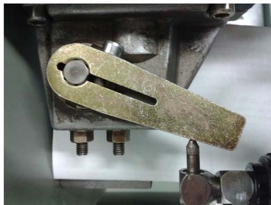
Figure 7 Position sensor measuring handle displacement
