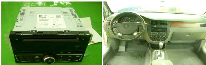
Picture 2. Installation process of Radio asm-am/fm stereo & audio disc player 92199291 is replaced radio with p/no. 42356100<sup>5</sup>
