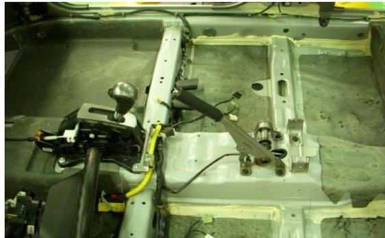
Picture 3. Installation process of Module asm-comn interface and nut communication interface is new added era-module with p/no. 94537398<sup>7</sup>
