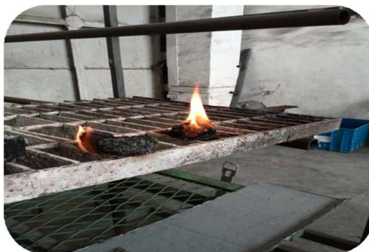
**Figure 6. Combustion of the fuel briquette.**
