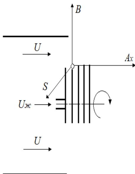
**Figure 1.** Scheme of installation of a pneumatic disc sprayer at the nozzle exit of the fan sprayer OVKh-600.
