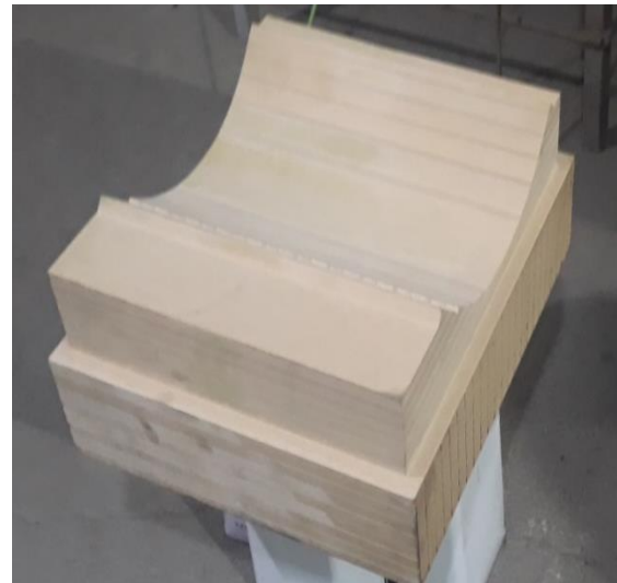
3-rasm. a). MDFdan quyma qolip shtamlash shtampi; b). Oldingi blok
