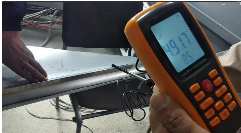
Fig.8. The air gap system is 5 mm and the distance to the saw tooth is 65 mm
