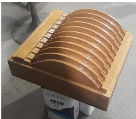
3-rasm. a). MDFdan quyma qolip shtamlash shtampi; b). Oldingi blok
