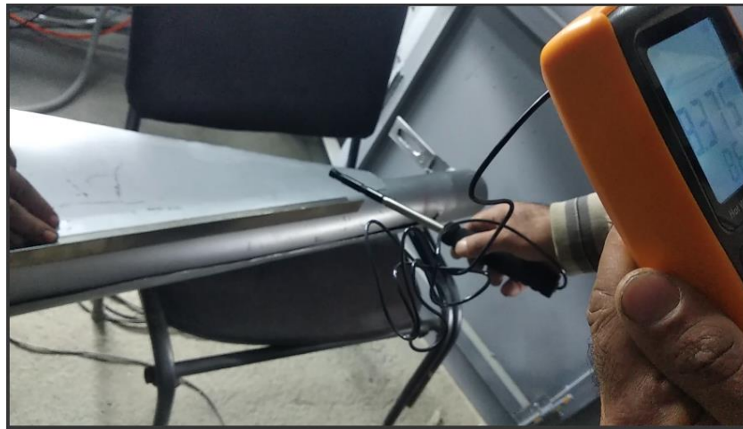
Fig.9. The air gap system is 5 mm and the distance to the saw tooth is 85 mm
