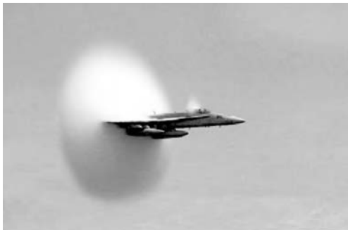
(c) Aircraft going through the sound barrier from subsonic to supersonic flight
