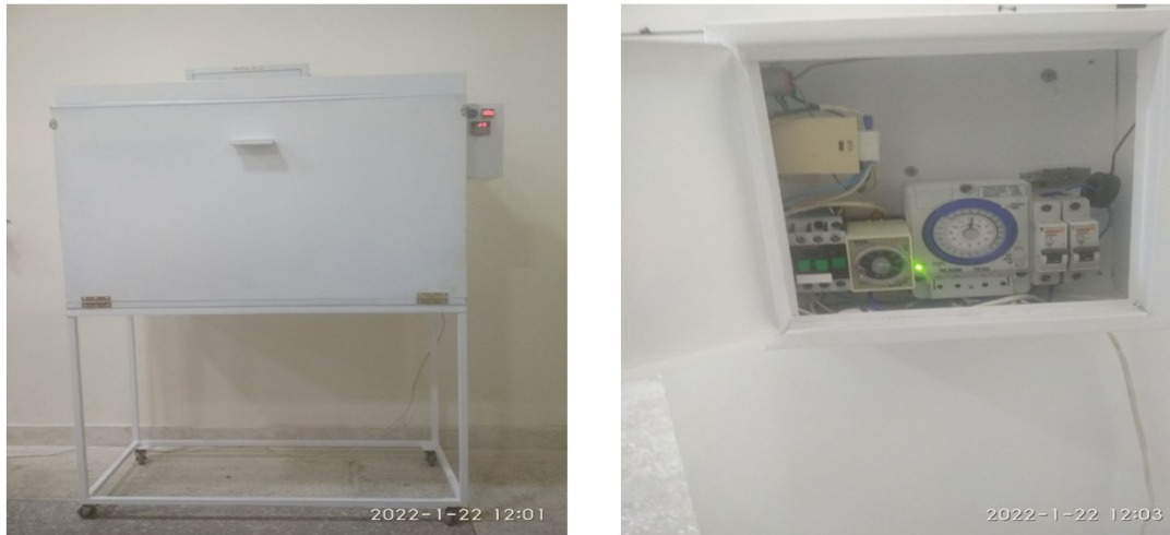
Figure 3. A device for irradiating sweet pepper seeds and irradiating seedlings and controlling the irradiation process.
