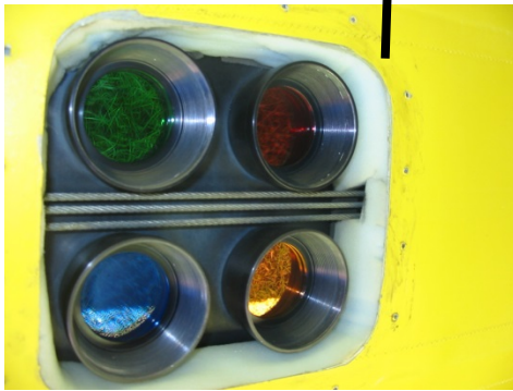
Multispectral camera system and GPS fitted to light aircraft
