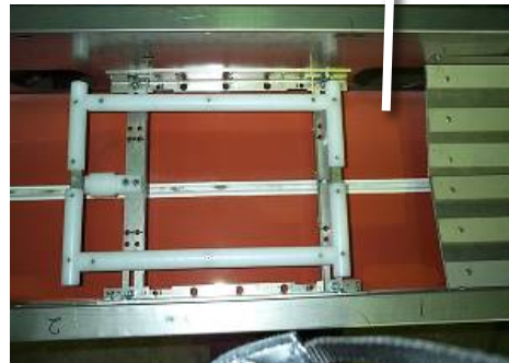
Weighing platform fitted to mechanical harvester
