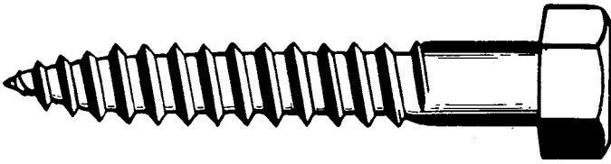
Figure I-22 Ordinary lag screw.
