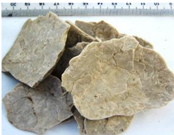
Figure 3. Micrograin limestone, tiled (Karakuduk 2 square, depth 3864 m).
