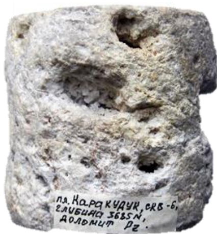
Figure 2. Cavernous secondary dolomite, sle. Karakuduk 6, int. 3685 m.
