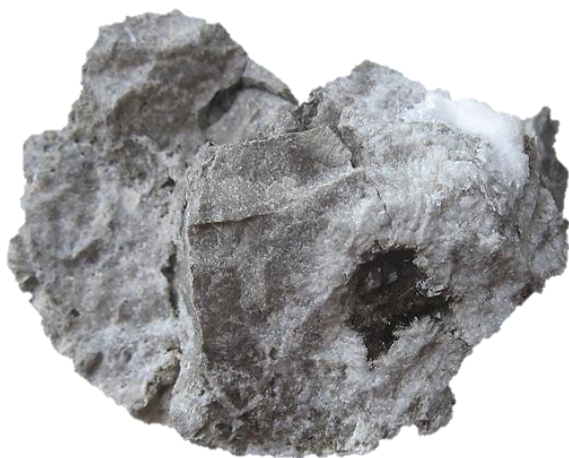
Figure 4. Kokchalak square 21, int. 3276-3280 m (C2-3). Oil priming along the dolomite caverns.
