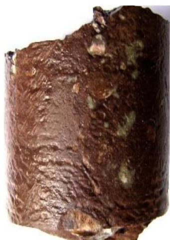
Figure 6. Sle. East Aituz-1. Brick-red clay siltstone, int. 3664.3-3675.0 m.
