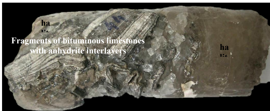
Figure 5. Fragments of clay limestones with layers of anhydrite in salts. Satbai-1, int. 1859 - 1866 m.
