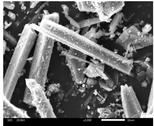
picture. 2. Microstructure of wollastonite fiber (x2000).
