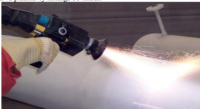
1-rasm. Gaz alangasida metallash
