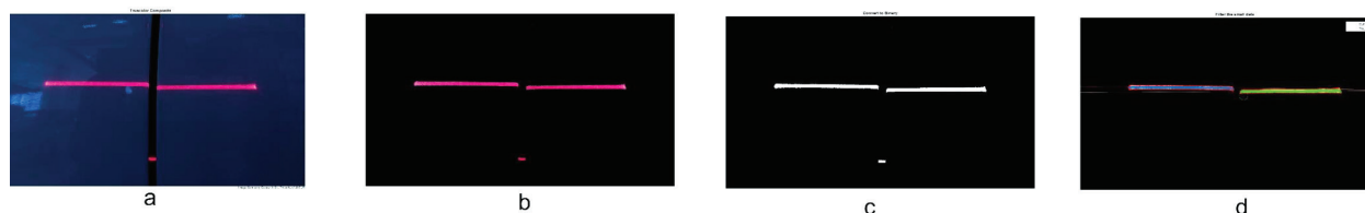
Figure 5. Image processing algorithm a) row color data b) extracted red c) binarized d) filtering and fitting is applied
