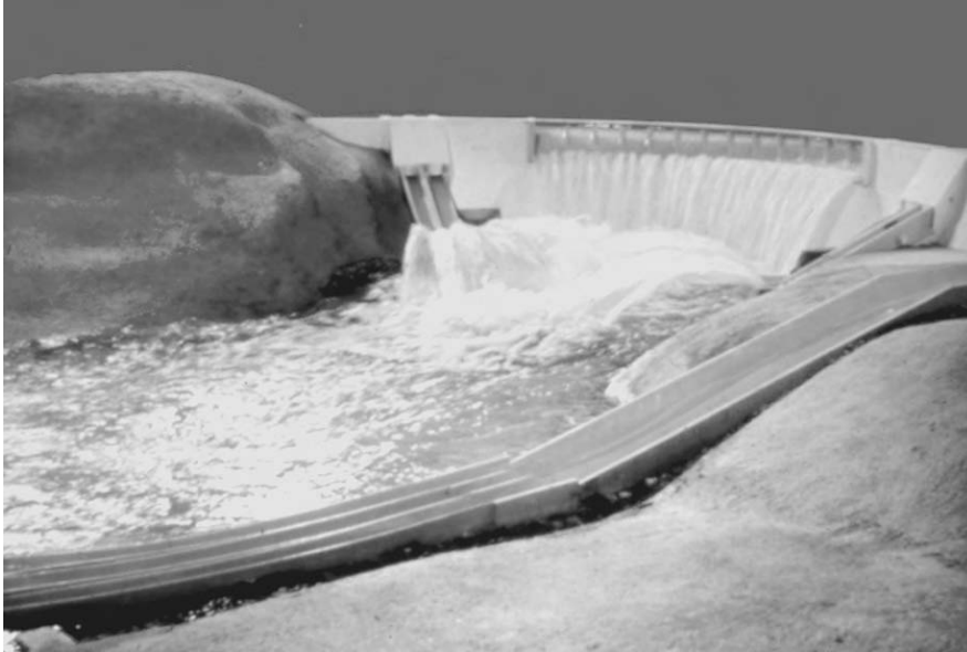
3.1 Laboratory model of a dam spillway.
