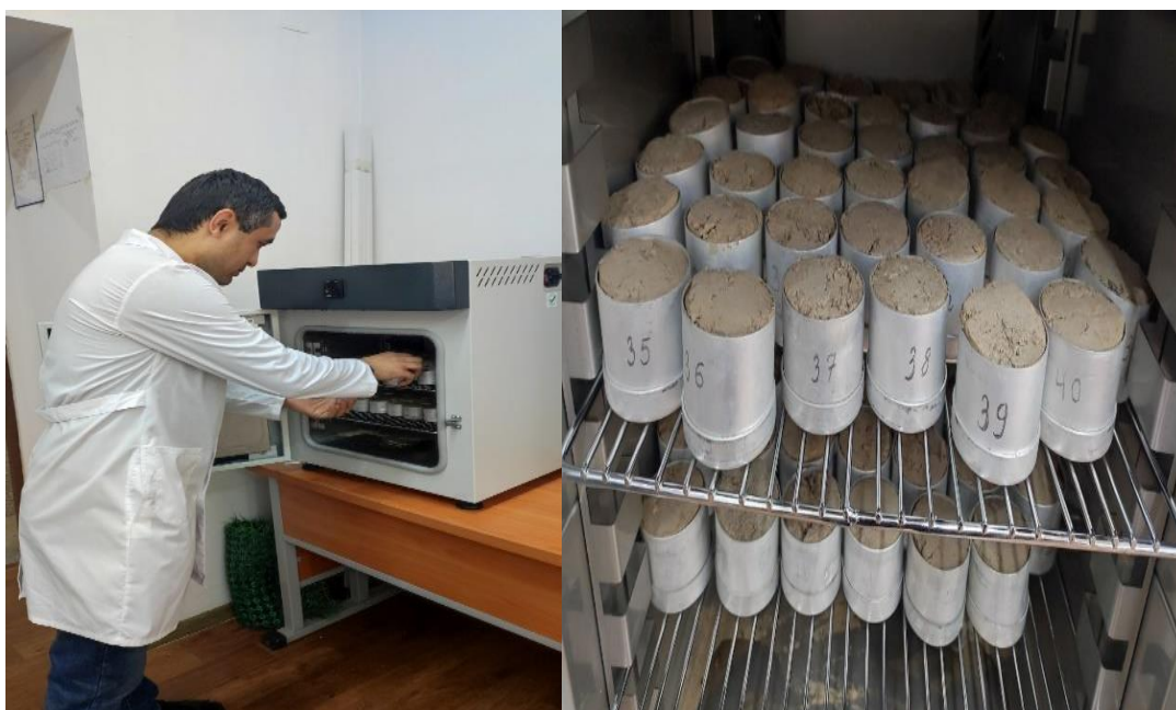
2.12-rasm. Tajriba maydonidan olingan tuproq namunalarini laboratoriya sharoitida o'rganish
