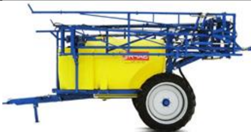
1.4-rasm. “Zarya” rusumli purkagichning tirkama varianti
