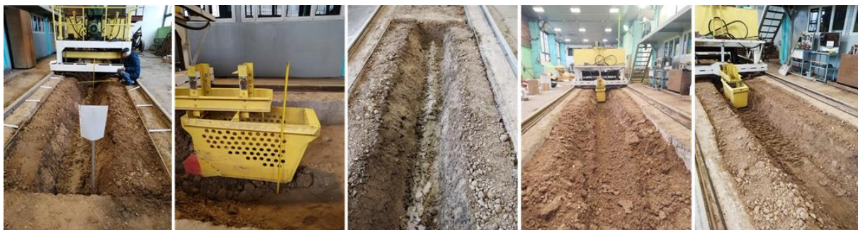
Figure 3. Laboratory tests of the bucket of the channel cleaner in actual size.
