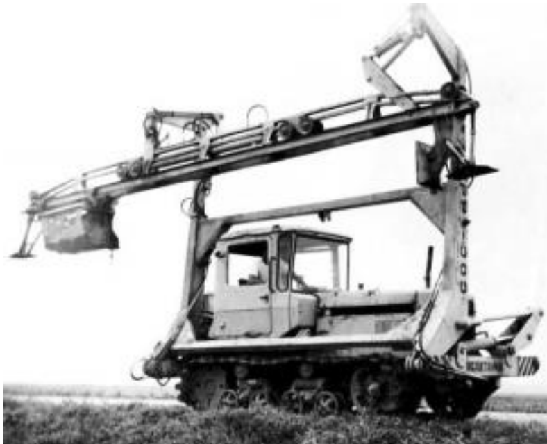
Figure 1. Channel cleaner with bucket on rigid guides.
