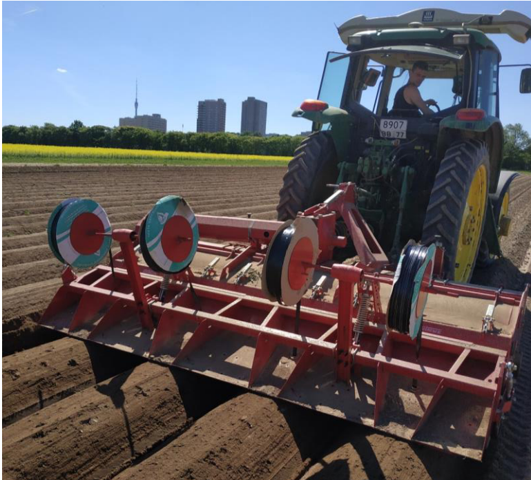
Fig. 4. Mechanized method using a Grimme GR-75/4 ridger modified for drip tape
